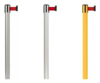
Choose from two grades of stainless steel or durable UPVC plastic. All posts are 63mm in diameter. Fixed in-floor installation using the aluminium slip post kit allows them to rotate for belt alignment while a security fixing prevents unauthorised removal. Available in a choice of six standard or four printed 3 metre belts with brake feature and self-locking clips. Slip post kits sold separately.
